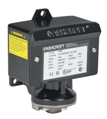
Ashcroft mechanical pressure switch, 4.5 to 30 psig set point, 0.5 to 1.5 psig deadband range, Buna-N sensing element, Buna-N seal(s), SPDT 15A, 1/4in female NPT process connection, 3/4in female NPT conduit opening.
