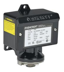
Ashcroft mechanical pressure switch, -30 to -4.5in Hg vacuum set point, 1.5 to 4.0in Hg deadband range, Buna-N sensing element, Buna-N seal(s), SPDT 15A, 1/4in female NPT process connection, 3/4in female NPT conduit opening.
