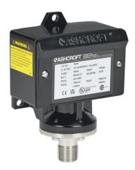
Ashcroft mechanical pressure switch, 450 to 3000 psig set point, 80 to 235 psig deadband range, Buna-N sensing element, Buna-N seal(s), SPDT 15A, 1/2in male NPT or 1/4in female NPT process connection, 3/4in female NPT conduit opening.
