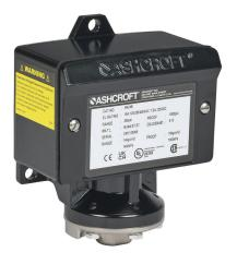
Ashcroft mechanical pressure switch, 30 to 200 psig set point, 5 to 13 psig deadband range, Buna-N sensing element, Buna-N seal(s), SPDT 15A, 1/4in female NPT process connection, 3/4in female NPT conduit opening.
