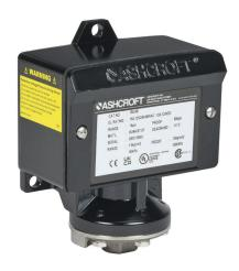
Ashcroft mechanical pressure switch, 2.25 to 15 psig set point, 0.5 to 1.5 psig deadband range, Buna-N sensing element, Buna-N seal(s), SPDT 15A, 1/4in female NPT process connection, 3/4in female NPT conduit opening.
