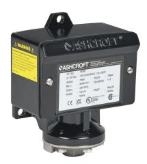
Ashcroft mechanical pressure switch, 15 to 100 psig set point, 1.5 to 5.0 psig deadband range, Buna-N sensing element, Buna-N seal(s), SPDT 15A, 1/4in female NPT process connection, 3/4in female NPT conduit opening.
