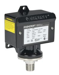
Ashcroft mechanical pressure switch, 150 to 1000 psig set point, 30 to 110 psig deadband range, Buna-N sensing element, Buna-N seal(s), SPDT 15A, 1/2in male NPT or 1/4in female NPT process connection, 3/4in female NPT conduit opening.
