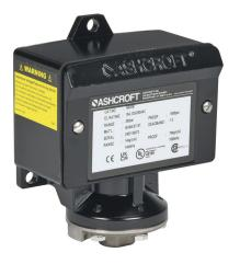
Ashcroft mechanical pressure switch, 30 to 200 psig set point, 1 to 3 psig deadband range, Buna-N sensing element, Buna-N seal(s), SPDT 15A, 1/4in female NPT process connection, 3/4in female NPT conduit opening.
