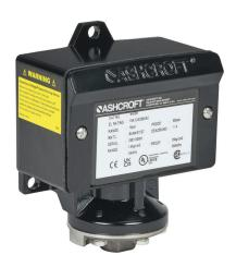
Ashcroft mechanical pressure switch, 2.25–15 psig set point, 0.1–0.35 psig deadband range, Buna-N sensing element, Buna-N seal(s), SPDT 15 A, 1/4 in female NPT process connection, 3/4 in female NPT conduit opening.
