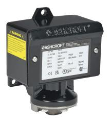
Ashcroft mechanical pressure switch, 15 to 100 psig set point, 0.5 to 1.7 psig deadband range, Buna-N sensing element, Buna-N seal(s), SPDT 15A, 1/4in female NPT process connection, 3/4in female NPT conduit opening.
