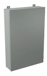
Wiegmann enclosure, NEMA 12, 36 x 24 x 7in (HxWxD), wall mount, carbon steel, ANSI 61 gray, powder coat finish, single-door, (3) plated steel clamps.
