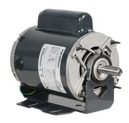
Marathon standard efficiency AC induction motor, fan and blower, 3/4hp, 1-phase, 115/208-230 VAC, 1800rpm, ODP, NEMA 56 frame, rolled steel, resilient base with extended studs mount.
