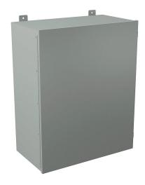
Wiegmann enclosure, NEMA 12, 30 x 24 x 13in (HxWxD), wall mount, carbon steel, ANSI 61 gray, powder coat finish, single-door, (2) plated steel clamps.
