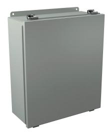
Wiegmann enclosure, NEMA 12/13, 16 x 14 x 6in (HxWxD), wall mount, carbon steel, ANSI 61 gray, powder coat finish, lift-off cover, (2) plated steel clamps.
