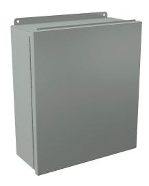
Wiegmann enclosure, NEMA 12/13, 16 x 14 x 6in (HxWxD), wall mount, carbon steel, ANSI 61 gray, powder coat finish, singledoor, (2) plated steel clamps.
