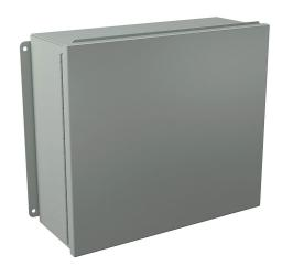
Wiegmann enclosure, NEMA 12/13, 14 x 16 x 6in (HxWxD), wall mount, carbon steel, ANSI 61 gray, powder coat finish, singledoor, (2) plated steel clamps.
