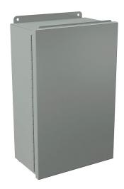
Wiegmann enclosure, NEMA 12/13, 16 x 10 x 6in (HxWxD), wall mount, carbon steel, ANSI 61 gray, powder coat finish, singledoor, (2) plated steel clamps.
