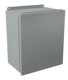
Wiegmann enclosure, NEMA 12/13, 14 x 12 x 8in (HxWxD), wall mount, carbon steel, ANSI 61 gray, powder coat finish, singledoor, (2) plated steel clamps.
