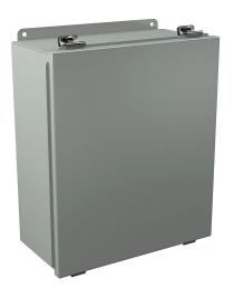
Wiegmann enclosure, NEMA 12/13, 14 x 12 x 6in (HxWxD), wall mount, carbon steel, ANSI 61 gray, powder coat finish, lift-off cover, (2) plated steel clamps.
