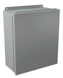
Wiegmann enclosure, NEMA 12/13, 14 x 12 x 6in (HxWxD), wall mount, carbon steel, ANSI 61 gray, powder coat finish, single-door, (2) quick-release latches.
