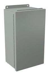
Wiegmann enclosure, NEMA 12/13, 14 x 8 x 6in (HxWxD), wall mount, carbon steel, ANSI 61 gray, powder coat finish, singledoor, (2) plated steel clamps.
