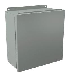
Wiegmann enclosure, NEMA 12/13, 12 x 12 x 6in (HxWxD), wall mount, carbon steel, ANSI 61 gray, powder coat finish, singledoor, (2) plated steel clamps.
