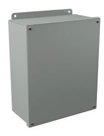
Wiegmann enclosure, NEMA 12/13, 12 x 10 x 5in (HxWxD), wall mount, carbon steel, ANSI 61 gray, powder coat finish, screw cover.
