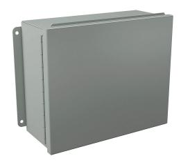
Wiegmann enclosure, NEMA 12/13,  $10 \times 12 \times 5$ in (HxWxD), wall mount, carbon steel, ANSI 61 gray, powder coat finish, singledoor, (2) plated steel clamps.
