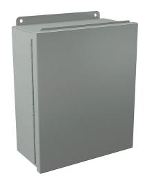
Wiegmann enclosure, NEMA 12/13, 12 x 10 x 5in (HxWxD), wall mount, carbon steel, ANSI 61 gray, powder coat finish, singledoor, (2) quick-release latches.
