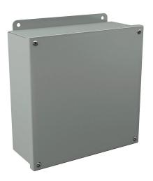
Wiegmann enclosure, NEMA 12/13, 10 x 10 x 4in (HxWxD), wall mount, carbon steel, ANSI 61 gray, powder coat finish, screw cover.
