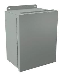
Wiegmann enclosure, NEMA 12/13, 10 x 8 x 6in (HxWxD), wall mount, carbon steel, ANSI 61 gray, powder coat finish, single-door, (2) plated steel clamps.
