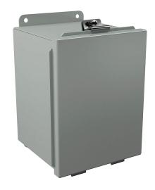
Wiegmann enclosure, NEMA 12/13, 8 x 6 x 6in (HxWxD), wall mount, carbon steel, ANSI 61 gray, powder coat finish, lift-off cover, (2) plated steel clamps.
