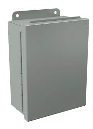
Wiegmann enclosure, NEMA 12/13, 8 x 6 x 3in (HxWxD), wall mount, carbon steel, ANSI 61 gray, powder coat finish, single-door, (2) plated steel clamps.
