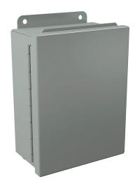
Wiegmann enclosure, NEMA 12/13, 8 x 6 x 3in (HxWxD), wall mount, carbon steel, ANSI 61 gray, powder coat finish, single-door, (2) quick-release latches.
