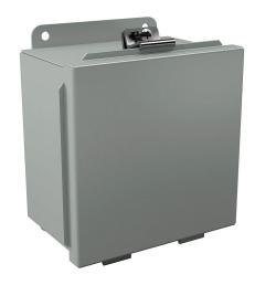
Wiegmann enclosure, NEMA 12/13, 6 x 6 x 4in (HxWxD), wall mount, carbon steel, ANSI 61 gray, powder coat finish, lift-off cover, (1) plated steel clamp.
