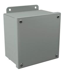
Wiegmann enclosure, NEMA 12/13, 6 x 6 x 4in (HxWxD), wall mount, carbon steel, ANSI 61 gray, powder coat finish, screw cover.
