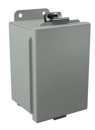
Wiegmann enclosure, NEMA 12/13, 6 x 4 x 4in (HxWxD), wall mount, carbon steel, ANSI 61 gray, powder coat finish, lift-off cover, (1) plated steel clamp.
