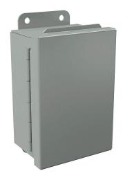
Wiegmann enclosure, NEMA 12/13, 6 x 4 x 3in (HxWxD), wall mount, carbon steel, ANSI 61 gray, powder coat finish, single-door, (1) plated steel clamp.
