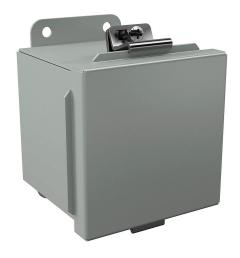
Wiegmann enclosure, NEMA 12/13, 4 x 4 x 4in (HxWxD), wall mount, carbon steel, ANSI 61 gray, powder coat finish, lift-off cover, (1) plated steel clamp.
