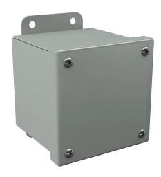
Wiegmann enclosure, NEMA 12/13, 4 x 4 x 4in (HxWxD), wall mount, carbon steel, ANSI 61 gray, powder coat finish, screw cover.
