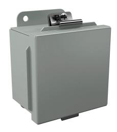
Wiegmann enclosure, NEMA 12/13, 4 x 4 x 3in (HxWxD), wall mount, carbon steel, ANSI 61 gray, powder coat finish, lift-off cover, (1) plated steel clamp.
