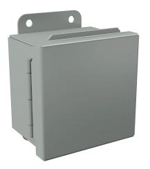
Wiegmann enclosure, NEMA 12/13,  $4 \times 4 \times 3$  in (HxWxD), wall mount, carbon steel, ANSI 61 gray, powder coat finish, single-door, (1) plated steel clamp.
