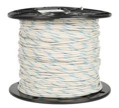
Atlas Wire AWM hook-up wire, single conductor, 26 AWG, 7-stranded, tinned copper, PVC conductor insulation material, white with blue stripe, 300V, 1000ft spool.
