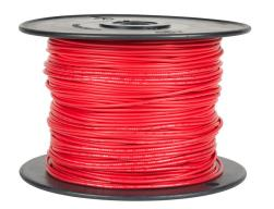
Atlas Wire AWM hook-up wire, single conductor, 26 AWG, 7-stranded, tinned copper, PVC conductor insulation material, red, 300V, 1000ft spool.
