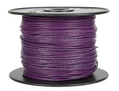
Atlas Wire AWM hook-up wire, single conductor, 26 AWG, 7-stranded, tinned copper, PVC conductor insulation material, purple, 300V, 1000ft spool.
