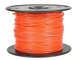
Atlas Wire AWM hook-up wire, single conductor, 26 AWG, 7-stranded, tinned copper, PVC conductor insulation material, orange, 300V, 1000ft spool.
