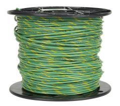
Atlas Wire AWM hook-up wire, single conductor, 26 AWG, 7-stranded, tinned copper, PVC conductor insulation material, green with yellow stripe, 300V, 1000ft spool.
