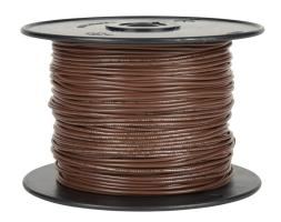
Atlas Wire AWM hook-up wire, single conductor, 26 AWG, 7-stranded, tinned copper, PVC conductor insulation material, brown, 300V, 1000ft spool.
