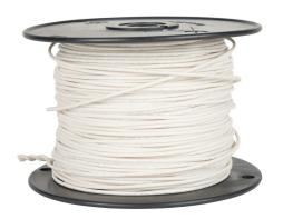
Atlas Wire AWM hook-up wire, single conductor, 24 AWG, 7-stranded, tinned copper, PVC conductor insulation material, white, 300V, 1000ft spool.
