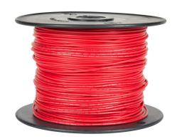
Atlas Wire AWM hook-up wire, single conductor, 24 AWG, 7-stranded, tinned copper, PVC conductor insulation material, red, 300V, 1000ft spool.
