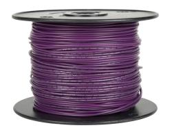
Atlas Wire AWM hook-up wire, single conductor, 24 AWG, 7-stranded, tinned copper, PVC conductor insulation material, purple, 300V, 1000ft spool.
