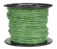
Atlas Wire AWM hook-up wire, single conductor, 24 AWG, 7-stranded, tinned copper, PVC conductor insulation material, green with yellow stripe, 300V, 1000ft spool.
