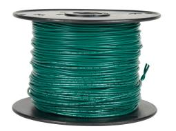
Atlas Wire AWM hook-up wire, single conductor, 24 AWG, 7-stranded, tinned copper, PVC conductor insulation material, green, 300V, 1000ft spool.
