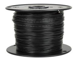
Atlas Wire AWM hook-up wire, single conductor, 24 AWG, 7-stranded, tinned copper, PVC conductor insulation material, black, 300V, 1000ft spool.
